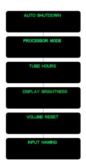
While a menu item is displayed, press 'ENTER', followed by rotating the volume knob on the front panel, or using the volume up/down buttons on the remote to adjust the settings of that particular selecton. After making the appropriate change, pressing the 'ENTER' button will confirm the new setting, and the display will show 'OKAY' for five seconds before reverting back to the normal operation screen.
